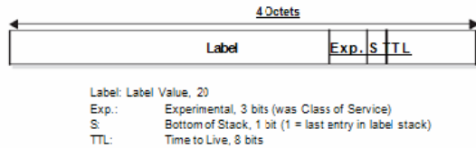
Figure 1.3 MPLS "shim" header format
